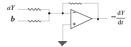
The constant term b is not related to any other term, it is a fixed potential. This can therefore be obtained from the power supply via an appropriate potential divider to give the value required.
