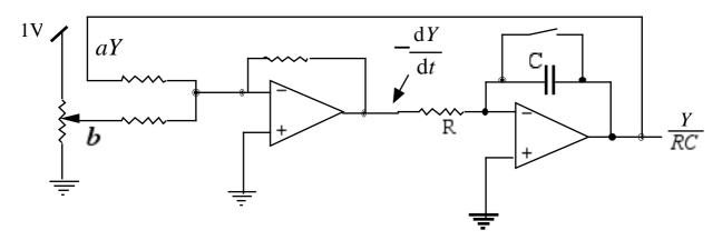
Note that the "solution" to the equation, Y, doesn't actually appear anywhere. The nearest to it is Y/RC, so if we want exactly Y we would need to include an additional amplifier or potential divider to scale this signal to give our final output.
