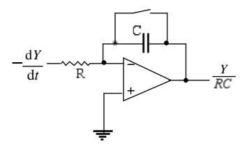
In practice the summer is an *inverting* circuit, but so is the integrator so these two inversions cancel out. So now we can connect up the entire circuit:
