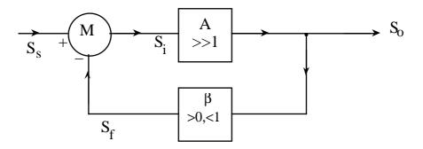
A is an amplifier with gain factor +A, and  $\beta$  is the feedback network which multiplies the output by the factor  $\beta$  (<1) before it is subtracted from the input to the circuit. "M" signifies the circuit element that subtracts the feedback from the input. If  $\beta$  (or A) is a negative number then the diagram will represent positive feedback.
