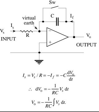
The output voltage is therefore the time-wise integral of the input signal. The time t=0 from which the integration begins – and at which the output voltage must be zero – is determined by holding the switch Sw closed until that instant. This switch can be a field-effect transistor (not available in *Crocodile Clips*), or for a slow circuit, a relay (electromagnetic switch).
