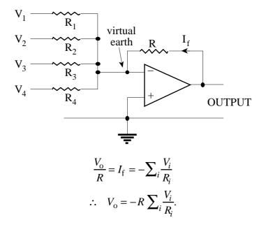
When all  $R_i = R$  then the output voltage is minus the sum of the input voltages.
