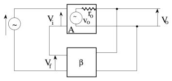
Then (taking  $V_s = 0$ ) the output current is  $I_o = (v_o - V_o)/r_o = (AV_i - V_o)/r_o = -(AV_f + V_o)/r_o = -(A\beta V_o + V_o)/r_o$  $= -(A\beta + 1)V_0/r_0$ .
