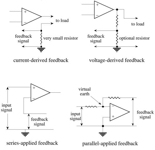
The resistor marked "optional" in the voltage-derived feedback circuit is not usually needed with parallel-applied feedback since the feedback current is determined by the other resistor alone.
