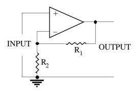
$\beta = R_2/(R_1 + R_2)$ , so the voltage gain is  $A_f = (R_1 + R_2)/R_2 = (1 + R_1/R_2)$ .
