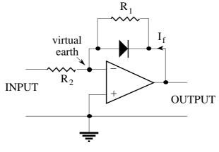
When the input is negative the output is positive and the diode is reverse biassed. The closed-loop gain is therefore  $-R_1/R_2$ .
