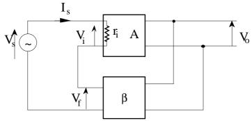
Let the amplifying element have an intrinsic input resistance  $r_i$ . Now the input current,
