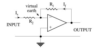
The standard NFB analysis, using a feedback factor  $\beta$ , would now have to be done in terms of feedback *current* and source *current*. However, we can avoid having to do this once we understand the operation of the *virtual earth*.
