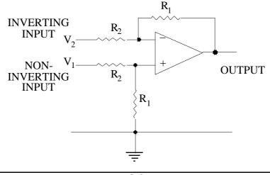
If we apply an input only at  $V_2$ , then  $V_1 = 0$  (i.e. earth), and the circuit is the same as the previous parallel-voltage feedback inverting amplifier with the addition of  $R_1$  and  $R_2$  in parallel between earth and the non-inverting input to the op amp. This makes no difference since there is a negligible current flowing into the op amp input. The closed loop-gain is therefore as before:
