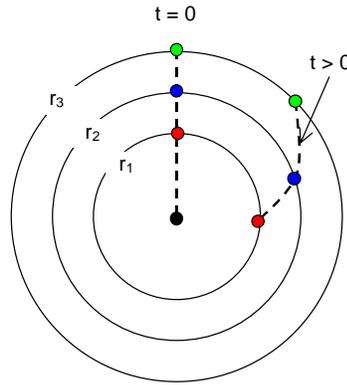
Figure 3-15. The origin of the winding problem.
