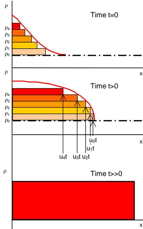
Figure 3-9. Development of a shock front.
