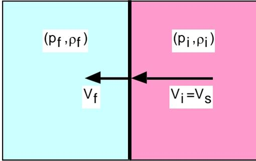
Figure 3-10. Frame of shock front.
