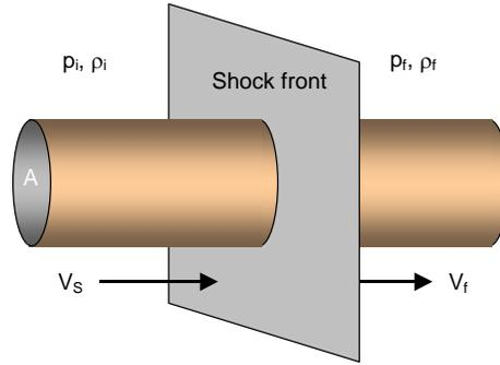
Figure 3-11. Material crossing shock front.
