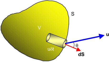
Figure 3-7, Flow of liquid.
